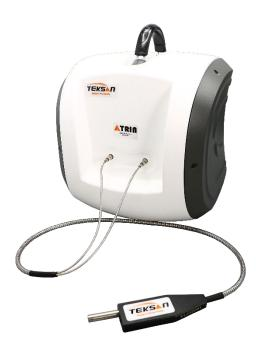
The development of portable Raman spectrometers has drastically changed the way the industry conducts quality control for incoming raw materials. Raman has always provided advantages over other methods in that it does not require sample pre-treatment or direct contact with the sample, and has the unique capability of being able to test a sample directly through a transparent packing material like glass or plastic.
